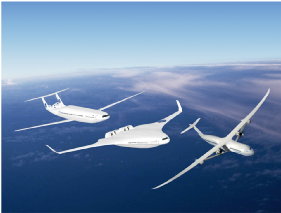
Figure 1. Conceptual illustration of fuel-efficient aircraft, including the truss-braced wing configuration (right), hybrid wing body configuration (center), and double-bubble configuration (left). Image credit: NASA.
